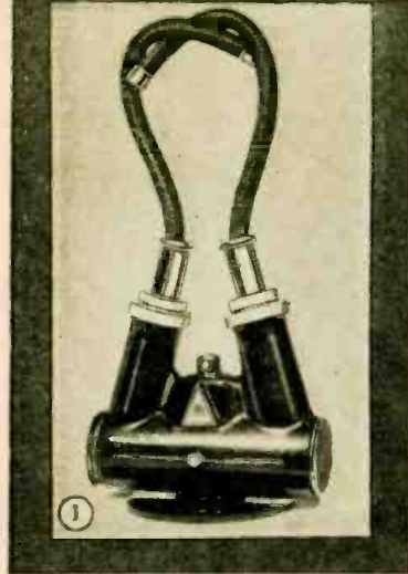
1—Therapeutic tube with shockproof shield. 2—Another shockproof tube for superficial therapy. 3—An air-cooled type—note the ventilating vanes. 4—Heavy rotating-anode X-ray tube.
